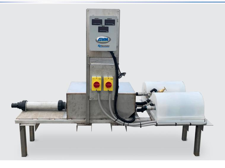
Accurately mixes up to three de-icing chemicals and allows users to quickly adapt to any weather event. Users can accurately reach any desired rate or effective temperature for their de-icing solutions using the GVM EZ Blend System.
